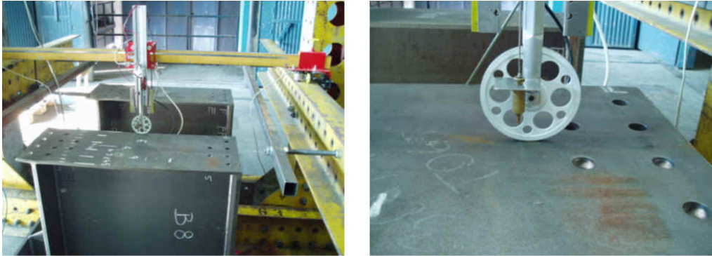
a.) specimens with the testing bar b.) measuring wheel with inductive transducer
